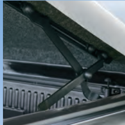
Scissor hinge provides a much improved fit
